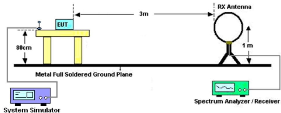
For radiated test from 30MHz to 1GHz
