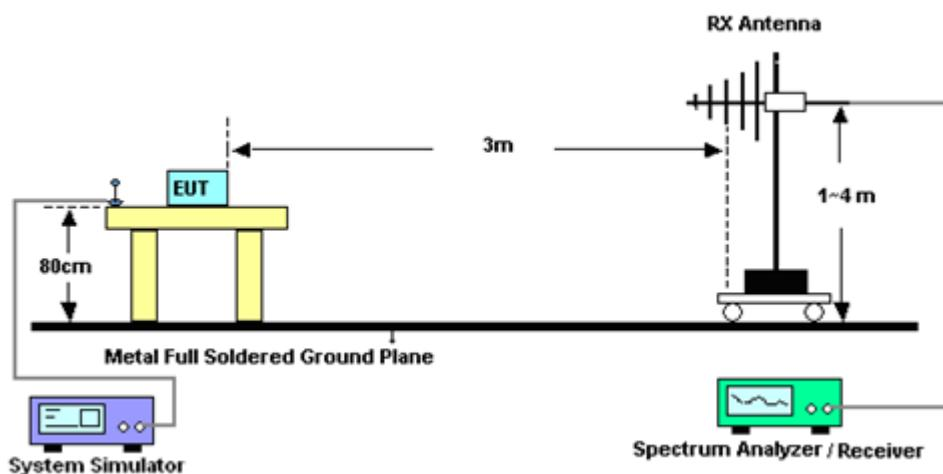
**For radiated test above 1GHz**
