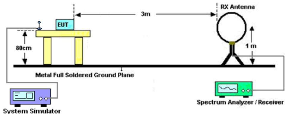
For radiated test from 30MHz to 1GHz
