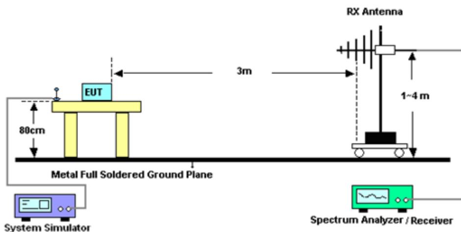
**For radiated test above 1GHz**
