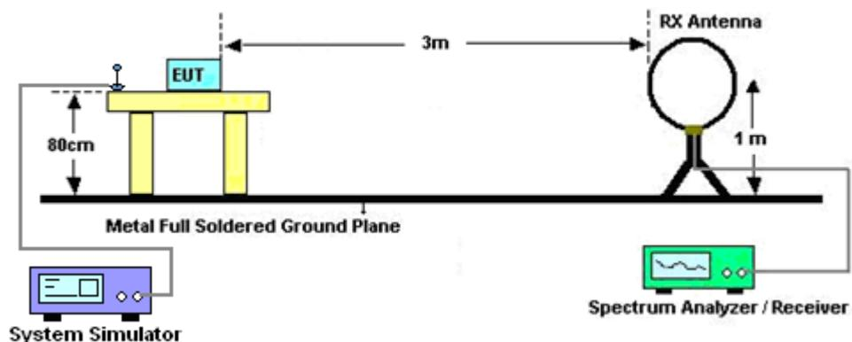
For radiated test from 30MHz to 1GHz
