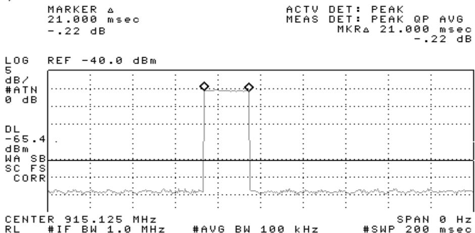
**Plot Showing Timing - duty cycle in any 100ms is 21ms/100ms, average correction factor is  $20\log(21/100) = -13.6\text{dB}$**
