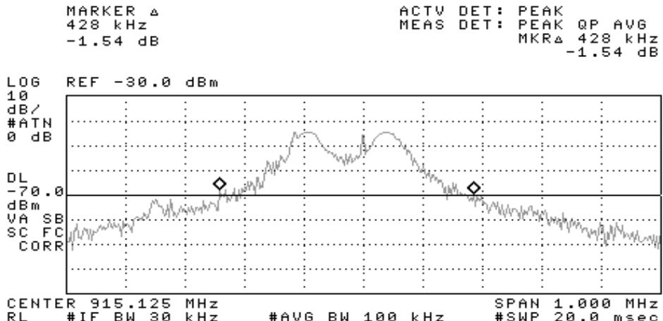
**Plot Showing Bandwidth - 26dB bandwidth = 428kHz**
