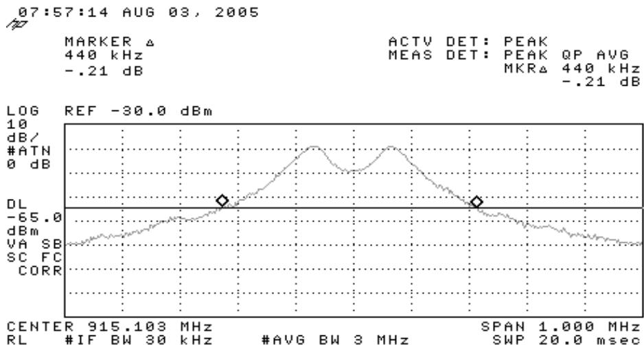
**Plot Showing Bandwidth - 26dB bandwidth = 440kHz**
