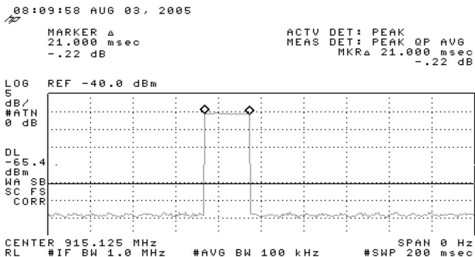
**Plot Showing Timing - duty cycle in any 100ms is 21ms/100ms, average correction factor is  $20\log(21/100) = -13.6\text{dB}$**
