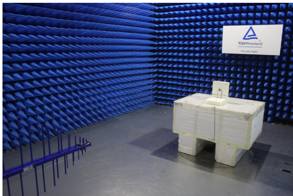
photograph of the setup, EUT in Charging mode in combination with AUX1
