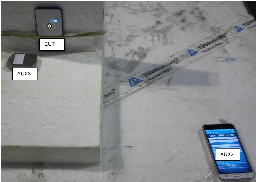
Photo 1a: EUT in a typical setup, Normal mode (during testing the AUX2 was placed as far away as possible from EUT and measurement antenna)
