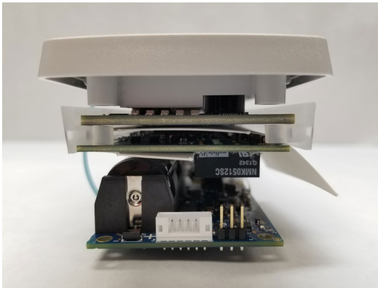
Figure 4 NIM Vital Patient Interface NIM4CPB1 Front View with Bottom Enclosure off
