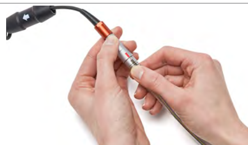
Figure 91: Pinch the grooved area of the controller Coiled Cable connector
