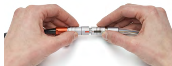
Figure 94: Push the connector into the port
