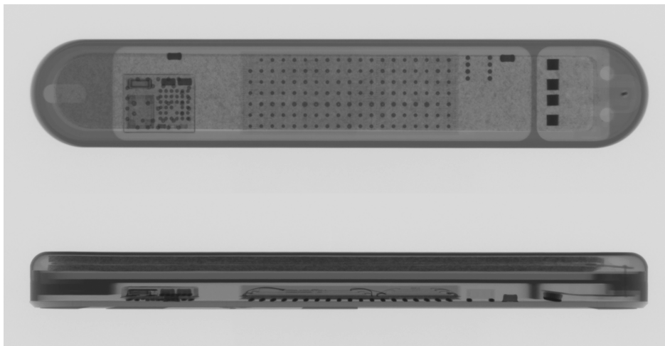
Figure 21. Front and side view X-ray images of an implanted LINQ II device
