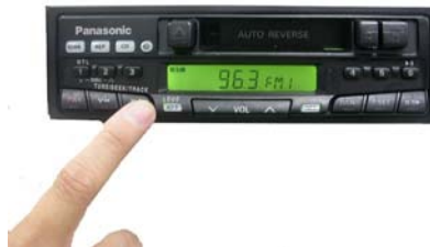
Pic-9 Adjust Radio frequency between 88Mhz~108Mhz
