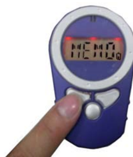
Pic-11 Set the selected channels to MEM0~MEM9
