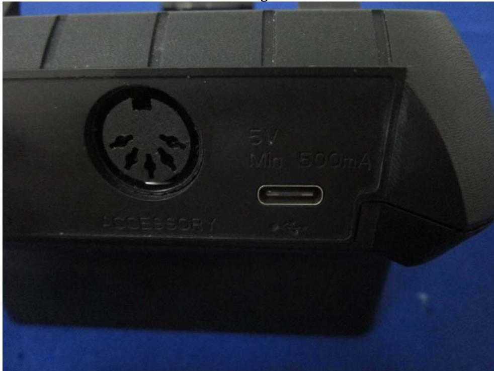
EUT – Base Charger Port View
