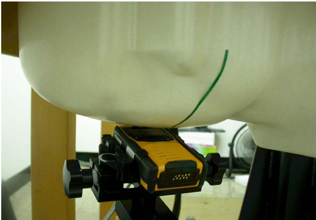
Measurement Position of Right-Tilt (RT) with Handset
