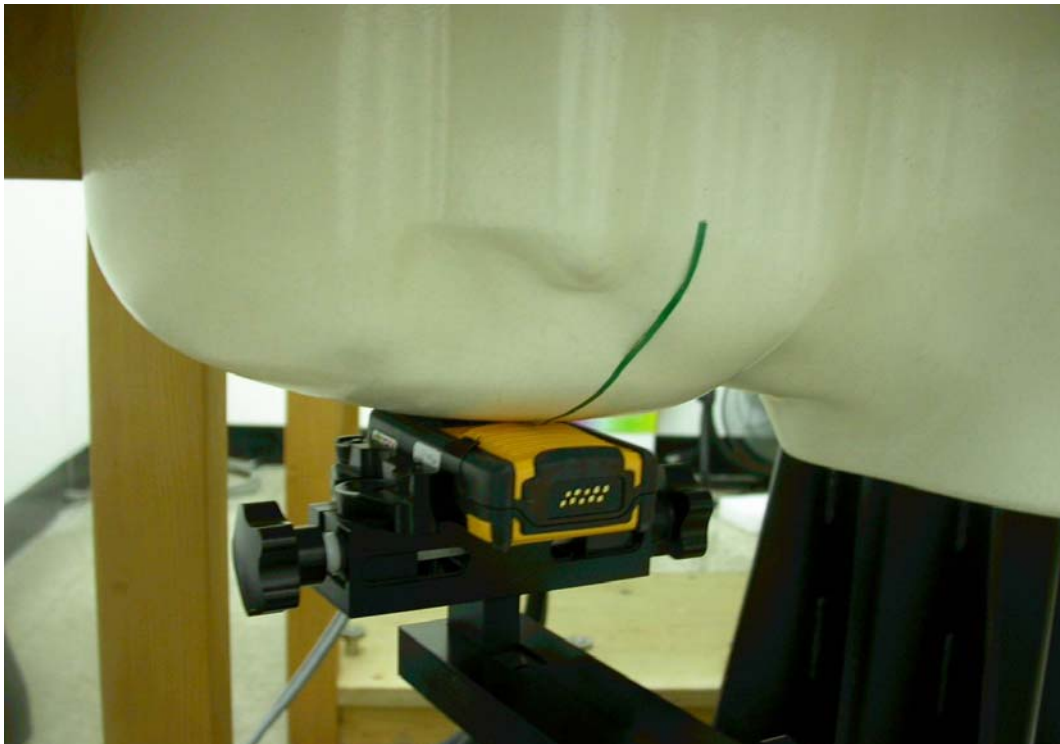
Measurement Position of Right-Cheek (RC) with Handset
