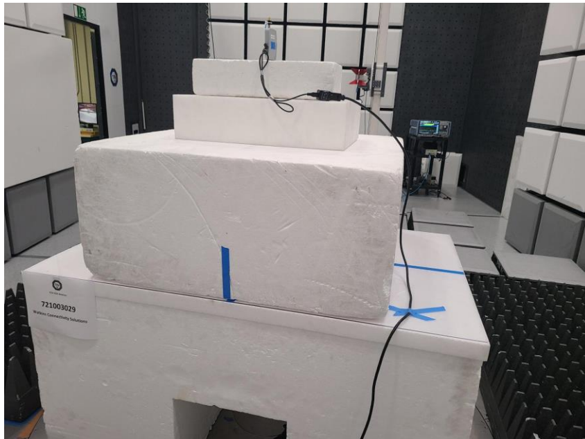
Radiated Emissions Test Setup (1GHz to 10GHz)
