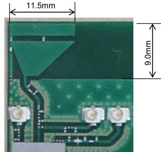
The 50ohm microstrip line and Type2EA\_Antenna needs to be copied when module is installed in the End product.
