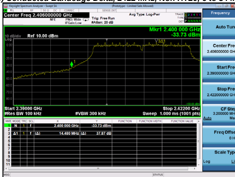
(-B) Conducted Bandedge Delta, 2412 MHz, Non HT20, 6 to 54 Mbps
