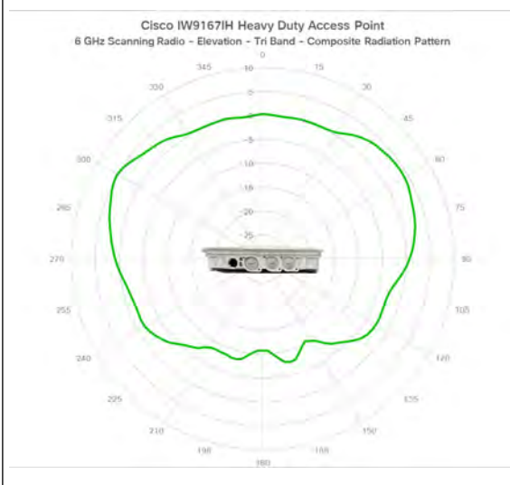
Figure 19: IW9167I - Scanning Radio - Tri Band Composite Radiation Pattern (6-GHz Elevation)
