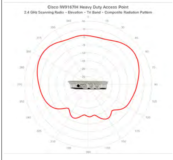
Figure 15: IW9167I - Scanning Radio-Tri Band Composite Radiation Pattern (2.4-GHz Elevation)
