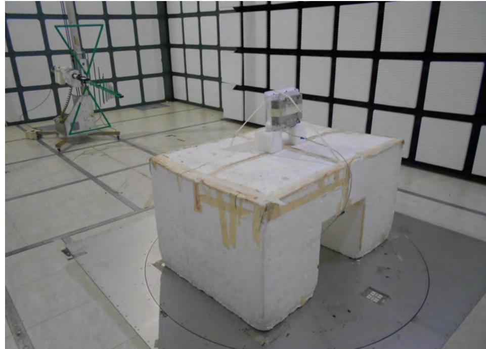
**Test Configuration: Above 1GHz / Test mode: Mode 1, 2, and 4**
