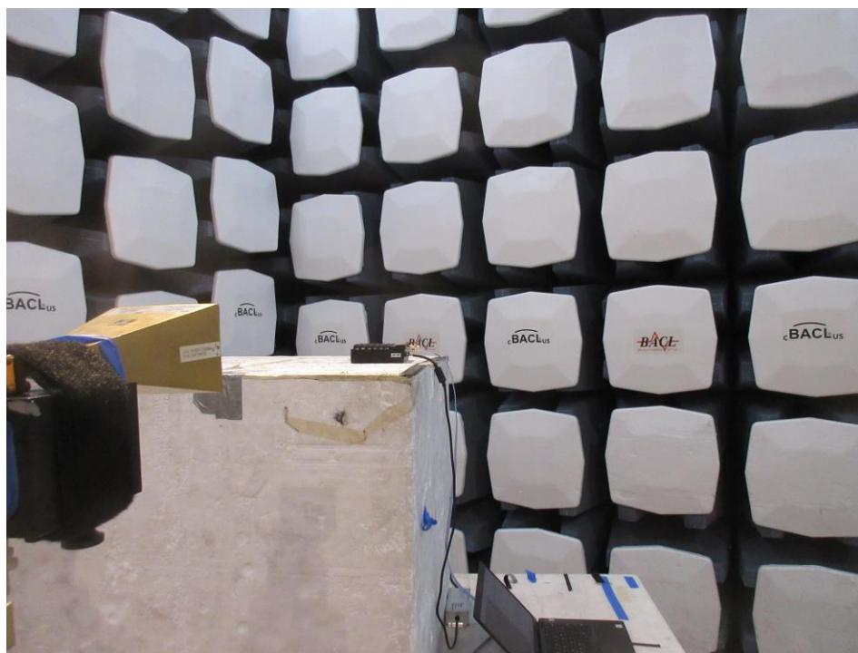
**1.8 Spurious Radiated Emissions: 18 GHz to 26.5 GHz, Rear View at 1 meter distance**
