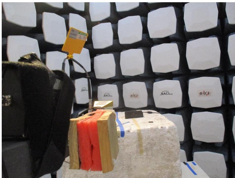
**1.10 Spurious Radiated Emissions: 26.5 GHz to 40 GHz, Rear View at 1 meter distance**
