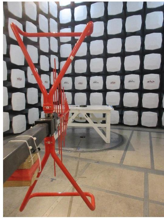
**1.4 Spurious Radiated Emissions: 30 MHz to 1000 MHz, Rear View at 3 meters distance**
