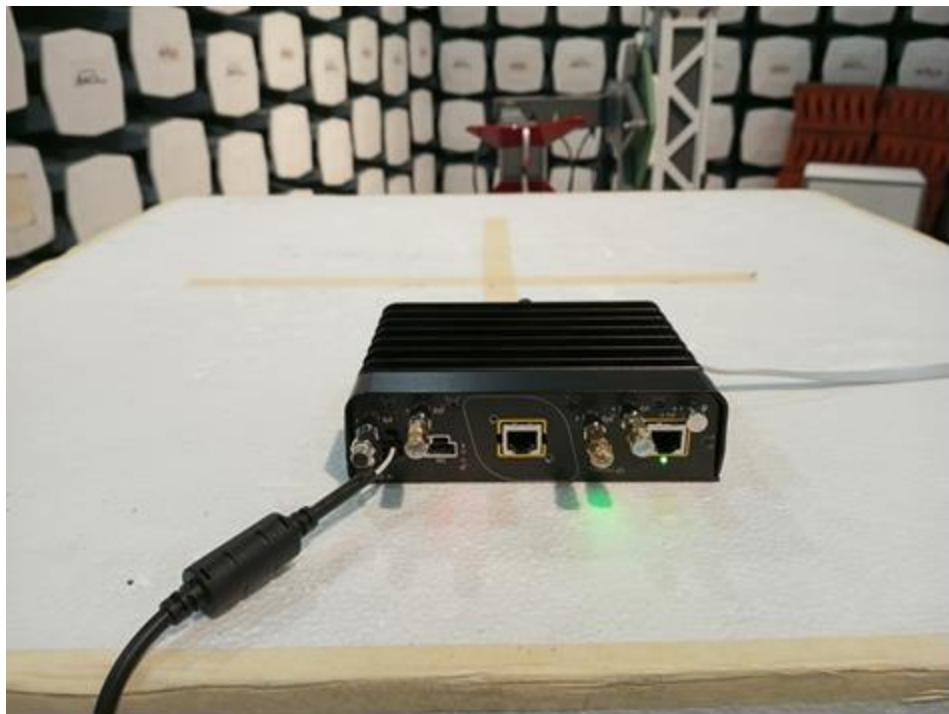
**1.7 Radiated Spurious Emissions: 18-26.5 GHz Front View at 1 meter**
