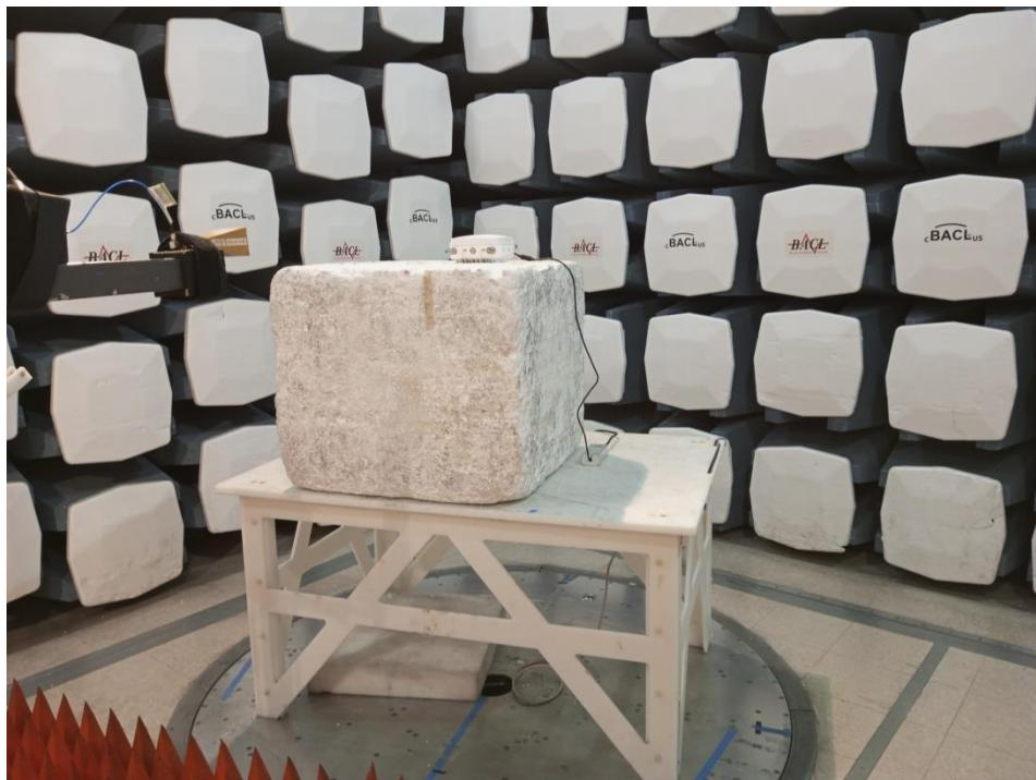
**1.8 Spurious Radiated Emissions: 26.5 GHz to 40 GHz, Rear View at 1 meter distance**
