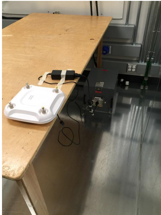
AIR-CAP3702P-B-K9 AC Conducted Emissions setup photo
