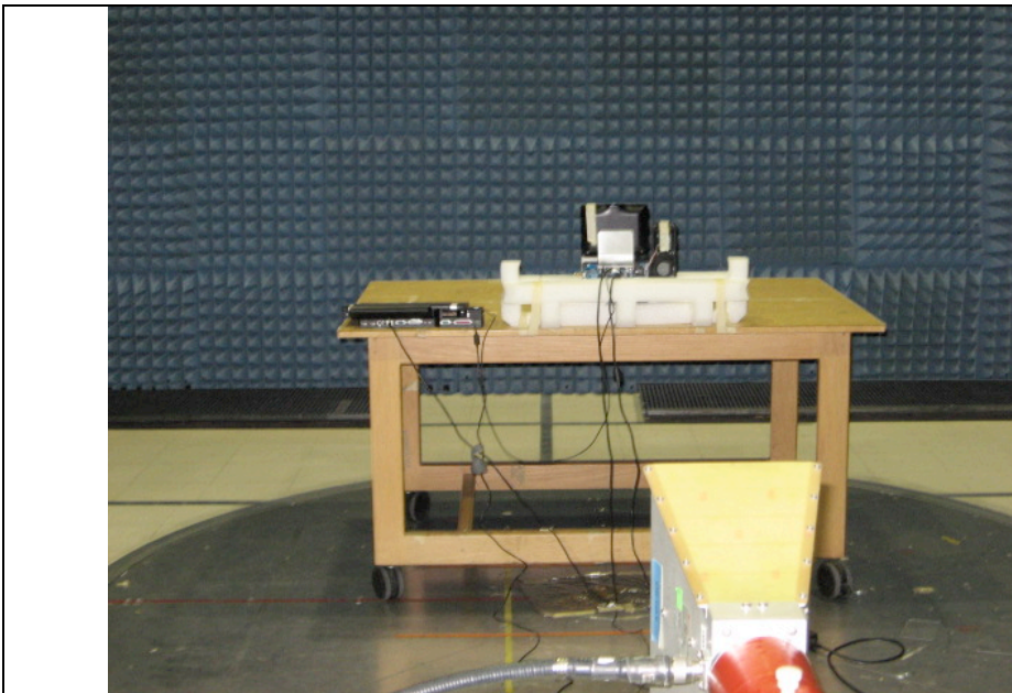
Title: Radiated Spurious Emissions 1 - 18GHz Test Setup
