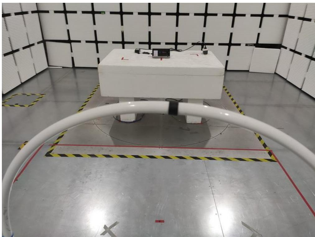
**Radiated Emissions Test Photos****30 MHz to 1000 MHz**
