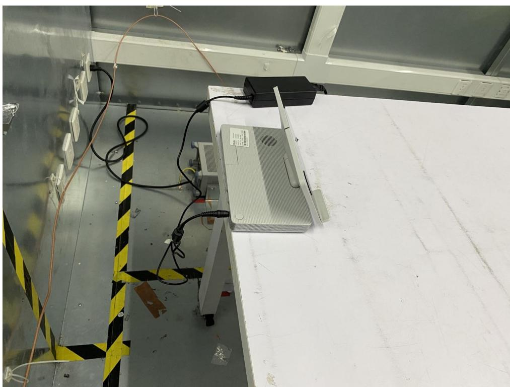
**Radiated Emissions Test Photos****9 kHz to 30 MHz**
