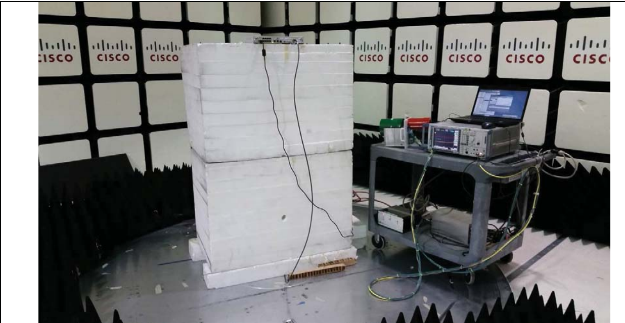
Title: Radiated Emissions Configuration Photograph 18-40GHz
