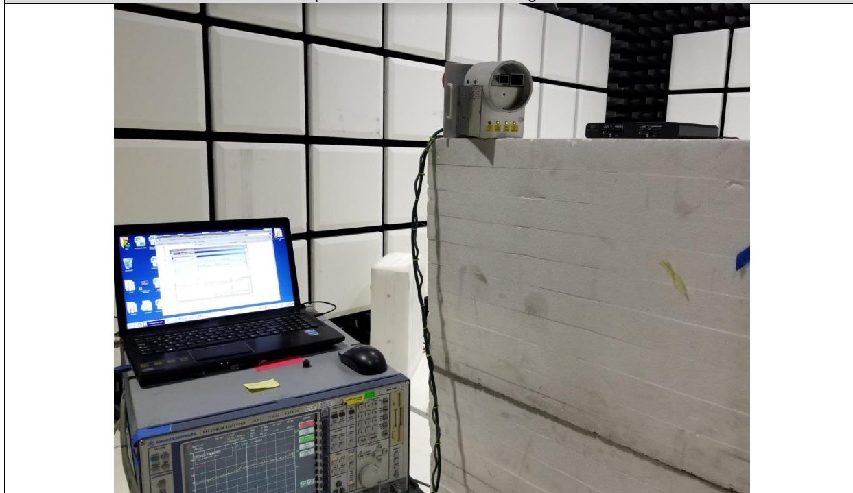
Title: Radiated Spurious Emissions Test Configuration 18 – 40GHz
