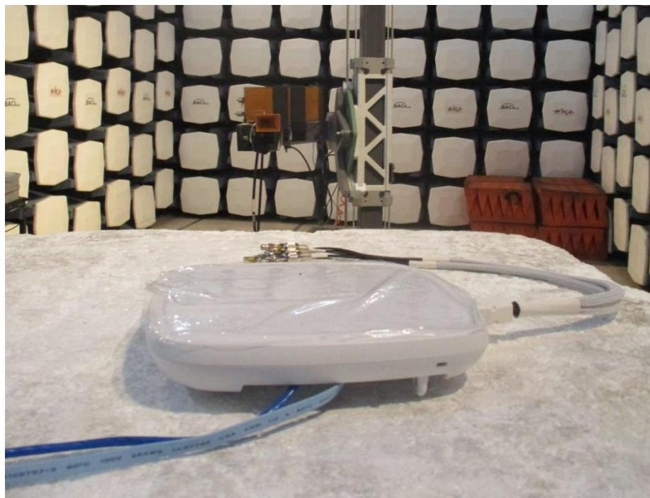
**1.8 Radiated Spurious Emission 26.5-40 GHz Rear View, 1 meter**
