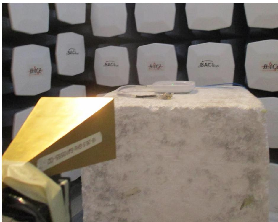
**1.7 Radiated Spurious Emission 26.5-40 GHz Front View, 1 meter**
