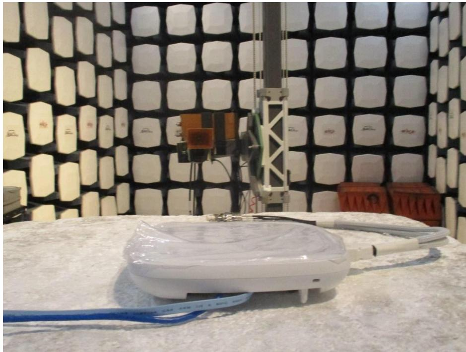
**1.6 Radiated Spurious Emission 18-26.5 GHz Rear View, 1 meter**
