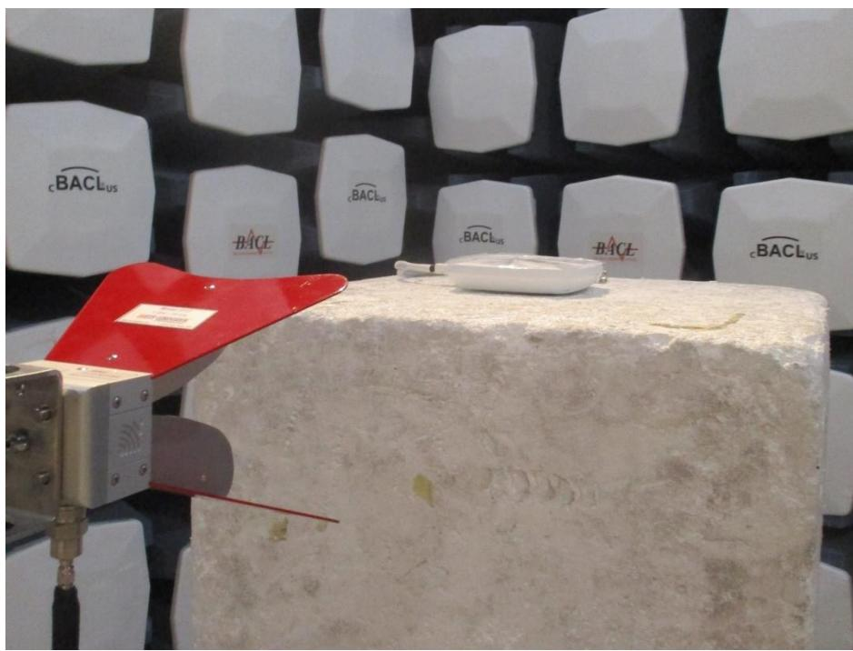
**1.5 Radiated Spurious Emission 18-26.5 GHz Front View, 1 meter**
