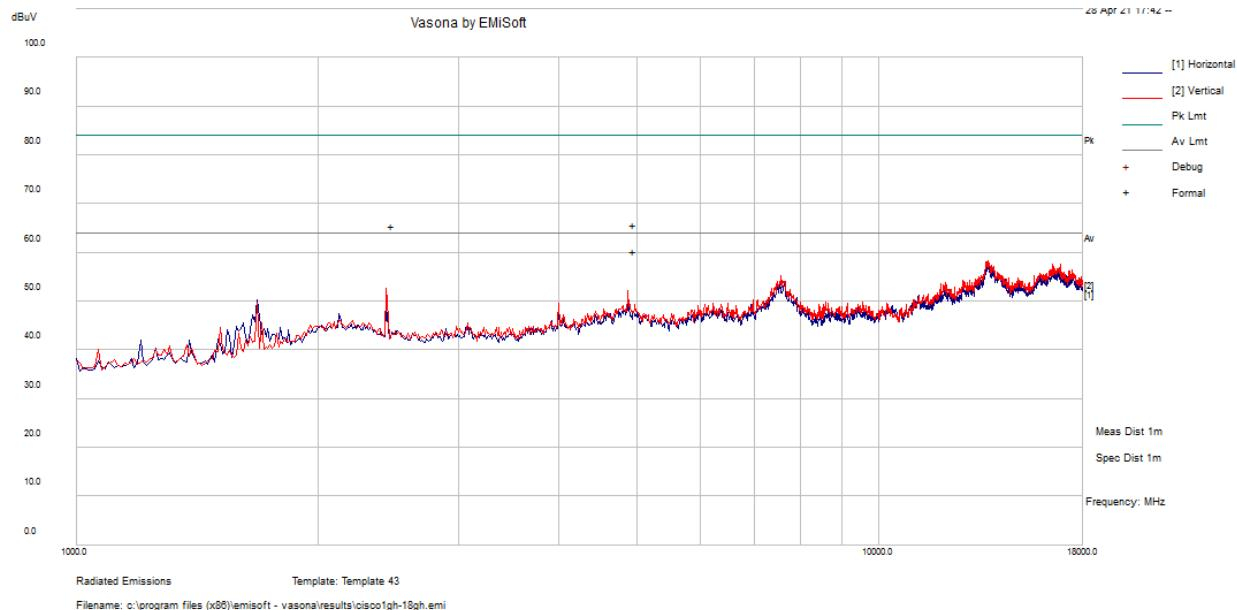
**3) 18 GHz-26.5 GHz, measured at 1 meter**
