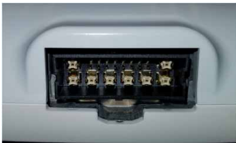
Figure 17 Smart Antenna Connector C9130AXE Model
