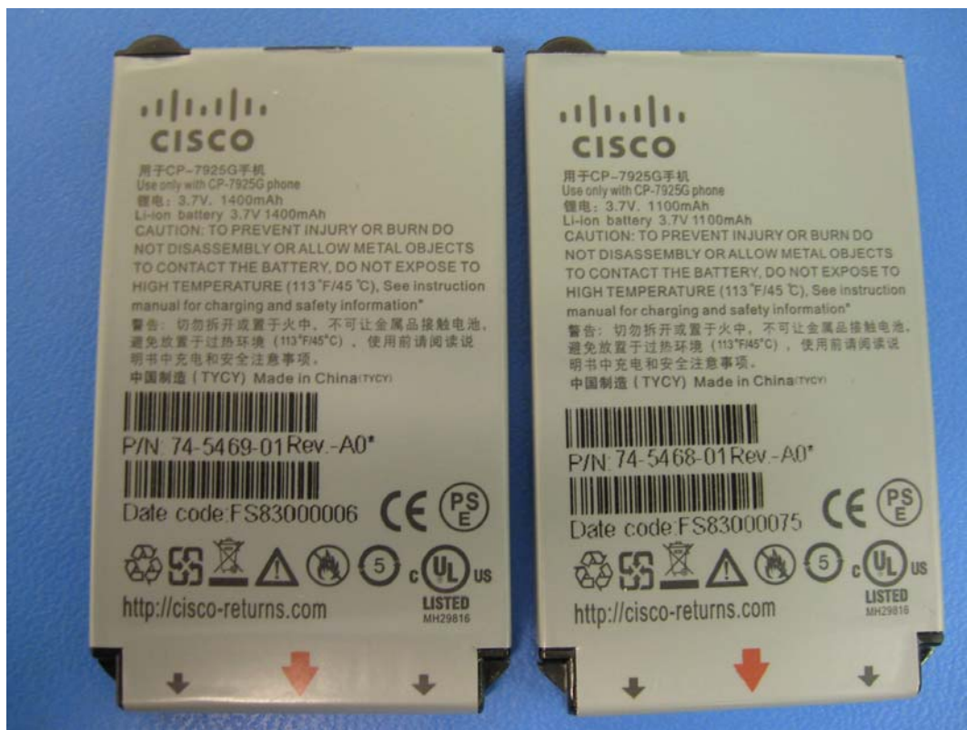
Standard and extended batteries inside View
