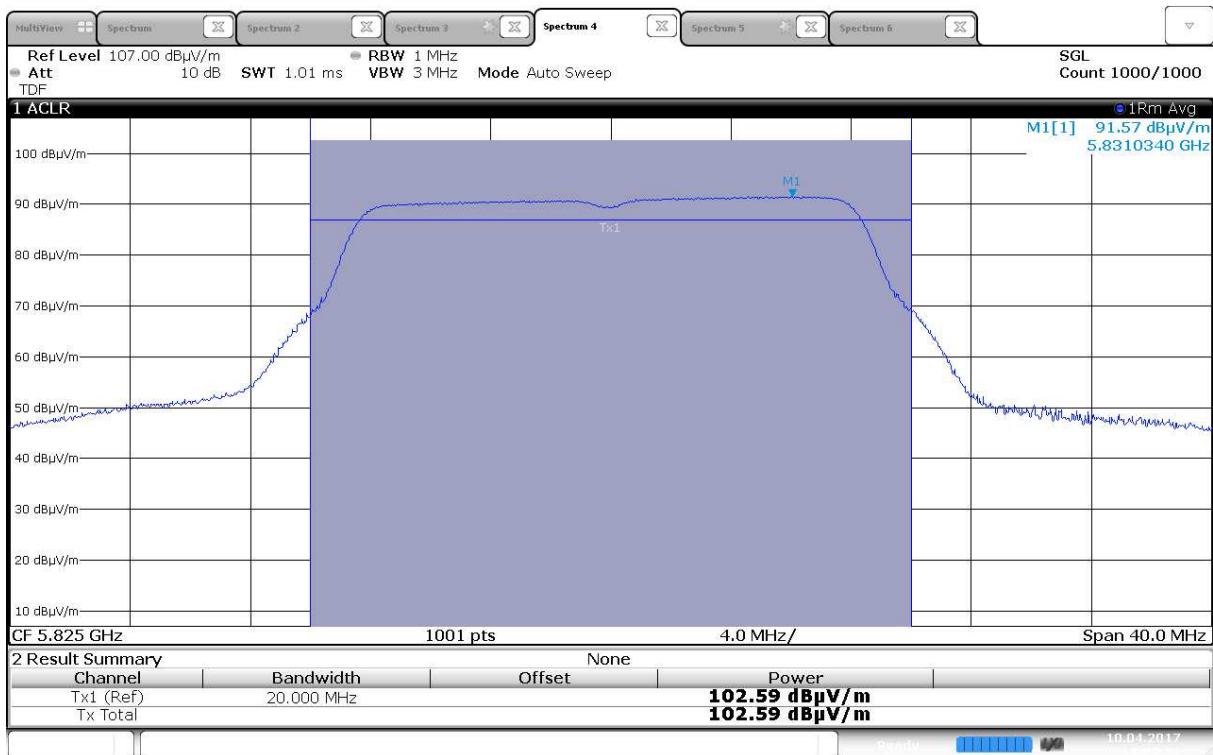
Maximum EIRP, 5825 MHz, 802.11a 6Mbps, Ant 1
