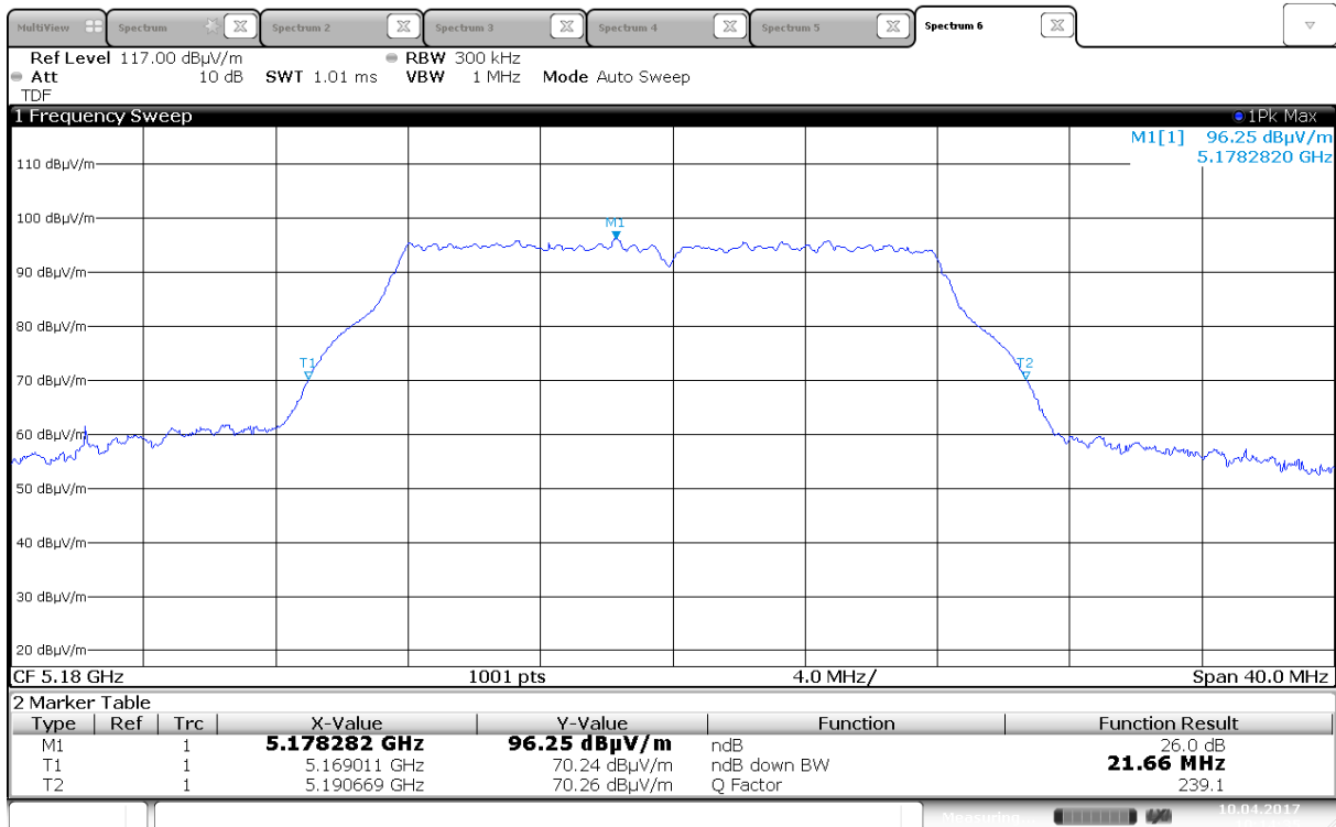
Emission Bandwidth B, 5180 MHz, 802.11a 6Mbps, Ant 1
