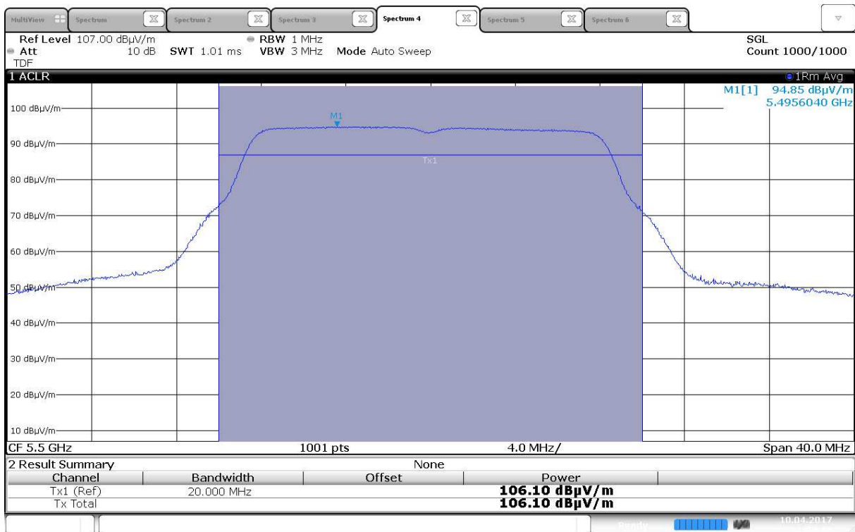
Maximum EIRP, 5500 MHz, 802.11a 6Mbps, Ant 1
