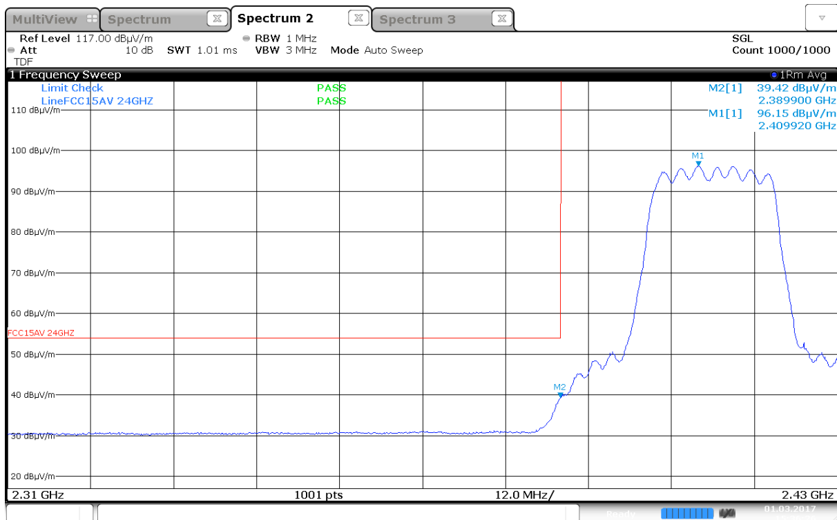
Lower Band Edge, Average, 2412 MHz, 802.11n, MCS0, (Max: Ant 0, HP)
