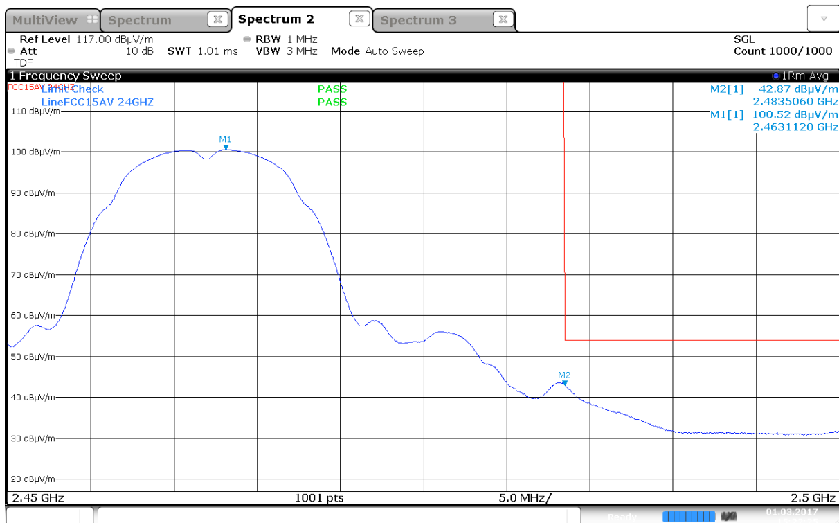
Upper Band Edge, Average, 2462 MHz, 802.11b, 1Mbps, (Max: Ant 0, HP)
