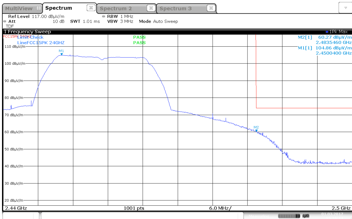
Upper Band Edge, Peak, 2457 MHz, 802.11g, 6Mbps, (Max: Ant 0, HP)
