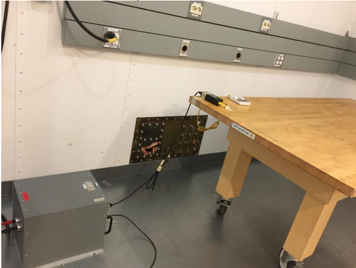
AC Mains Conducted Emissions setup
