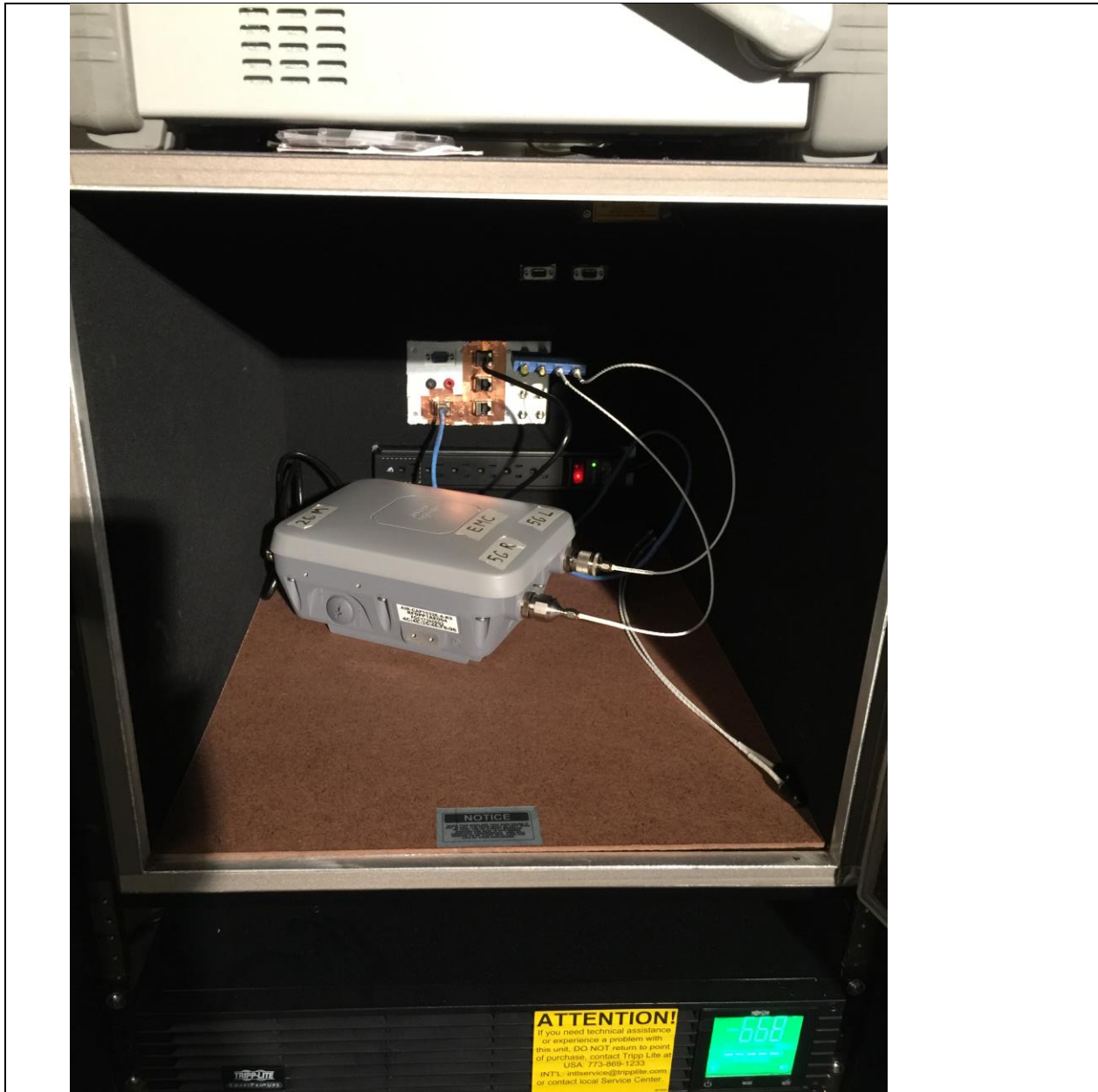
Title: AIR-CAP1532I-B-K9 Conducted Test Setup
