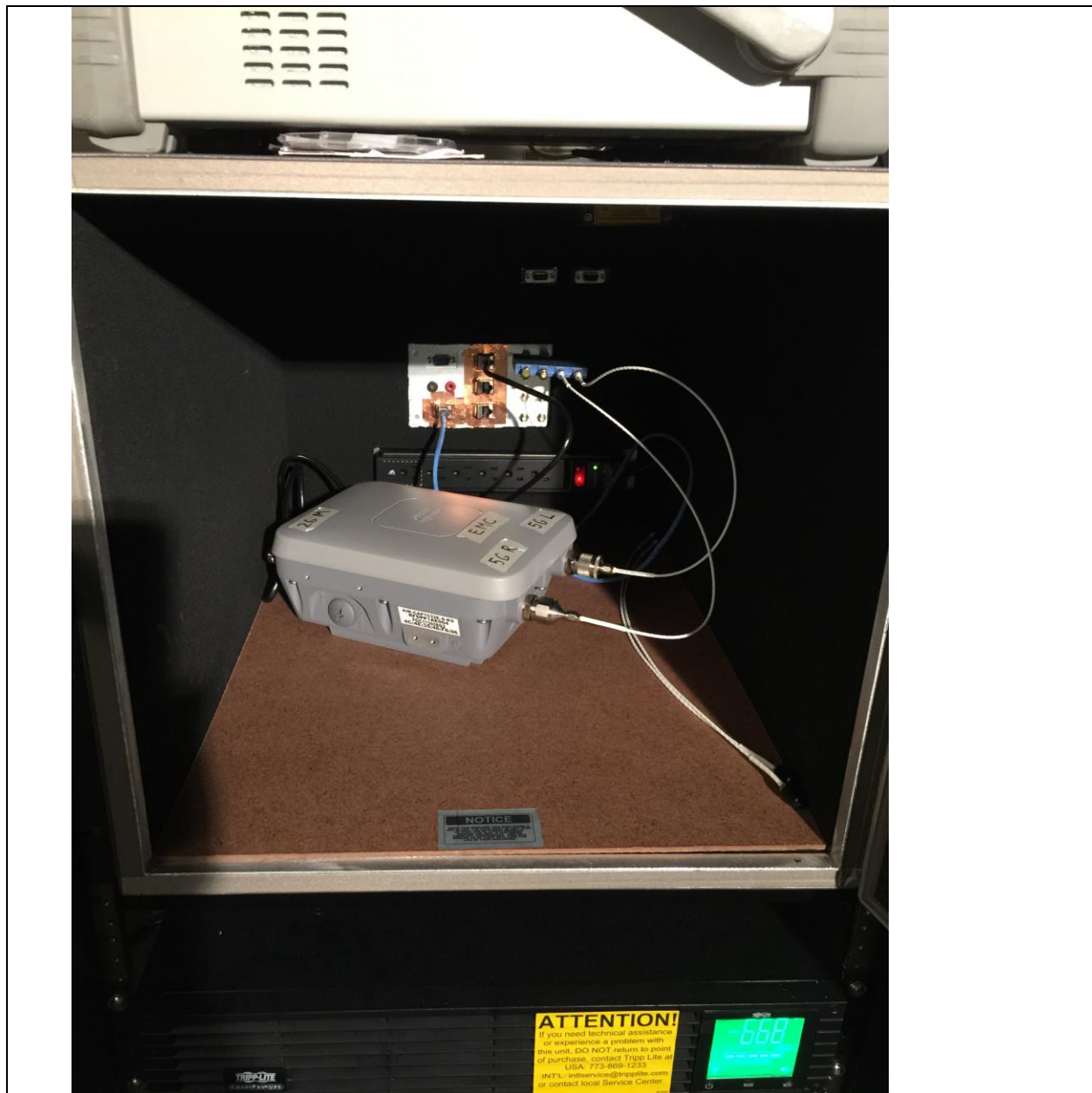
Title: AIR-CAP1532I-B-K9 Conducted Test Setup
