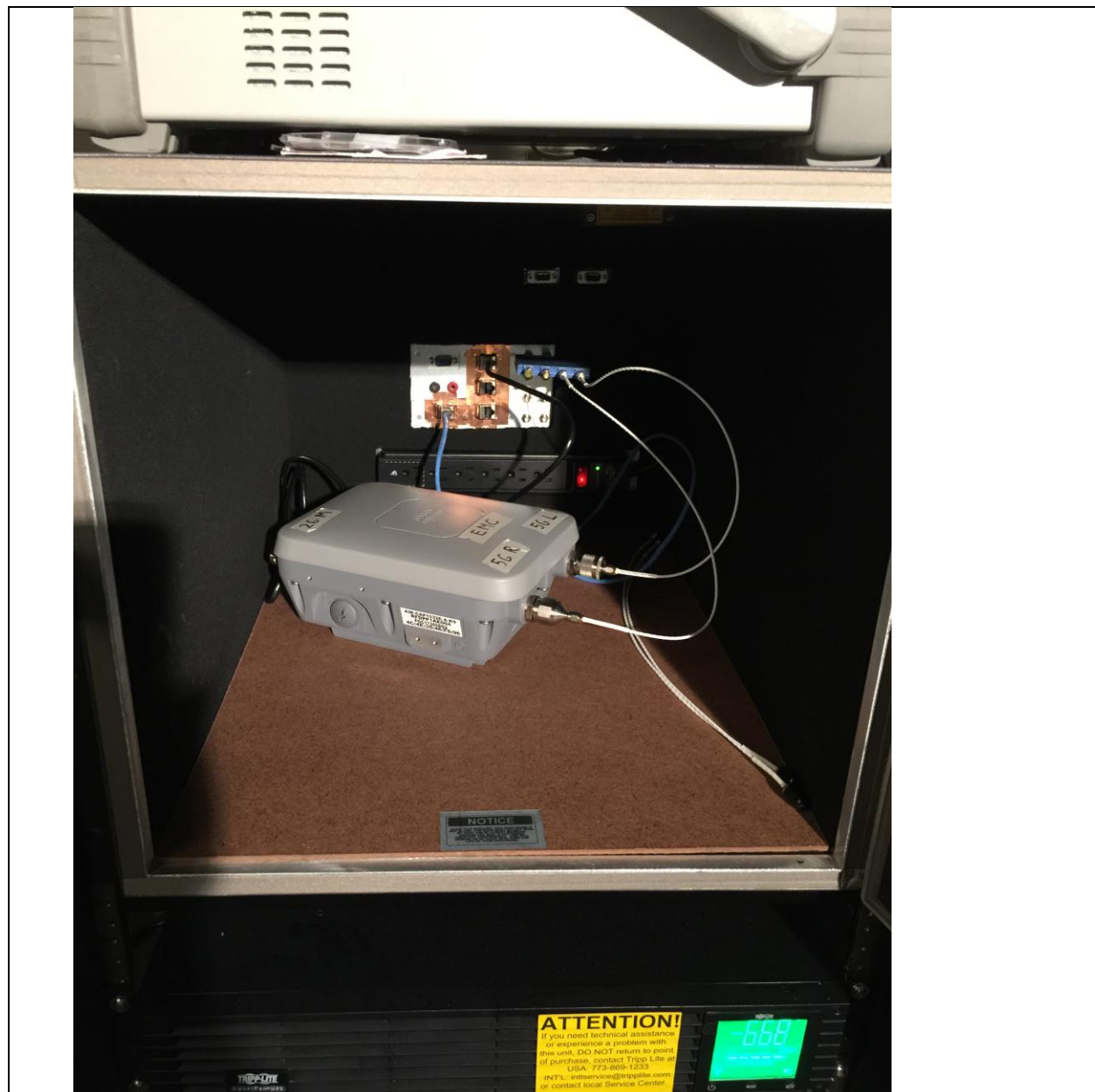
Title: AIR-CAP1532E-B-K9 Conducted Test Setup
