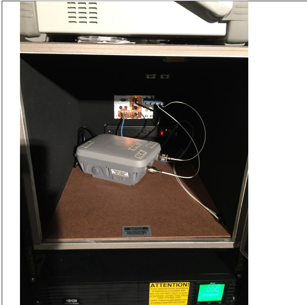
Title: AIR-CAP1532E-B-K9 Conducted Test Setup
