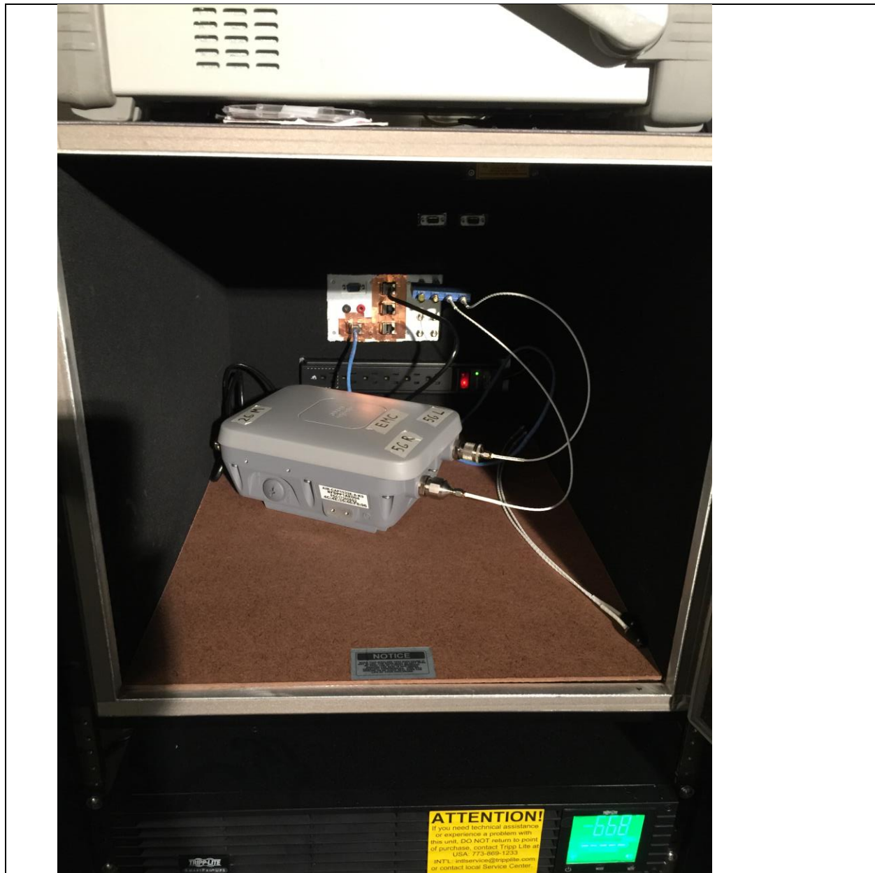
Title: AIR-CAP1532E-B-K9 Conducted Test Setup
