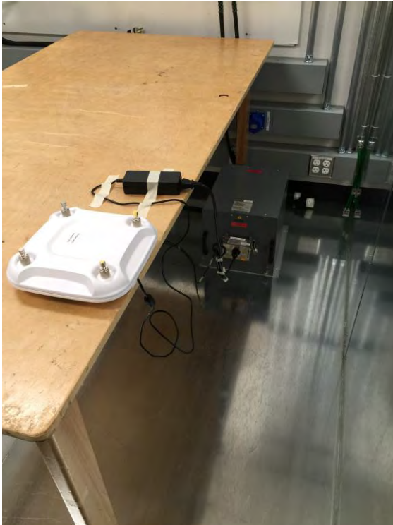
AIR-CAP3702P-B-K9 AC Conducted Emissions setup photo
