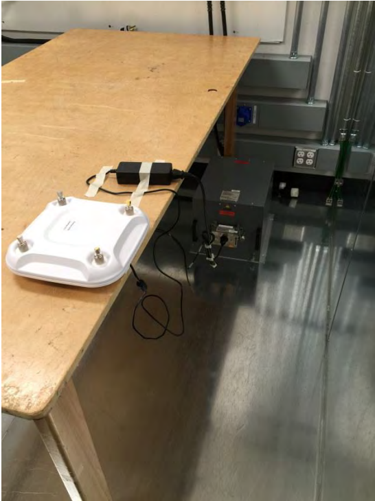
AIR-CAP3702P-B-K9 AC Conducted Emissions setup photo
