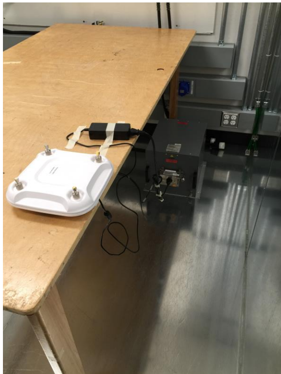
AIR-CAP3702E-B-K9 AC Conducted Emissions setup photo
