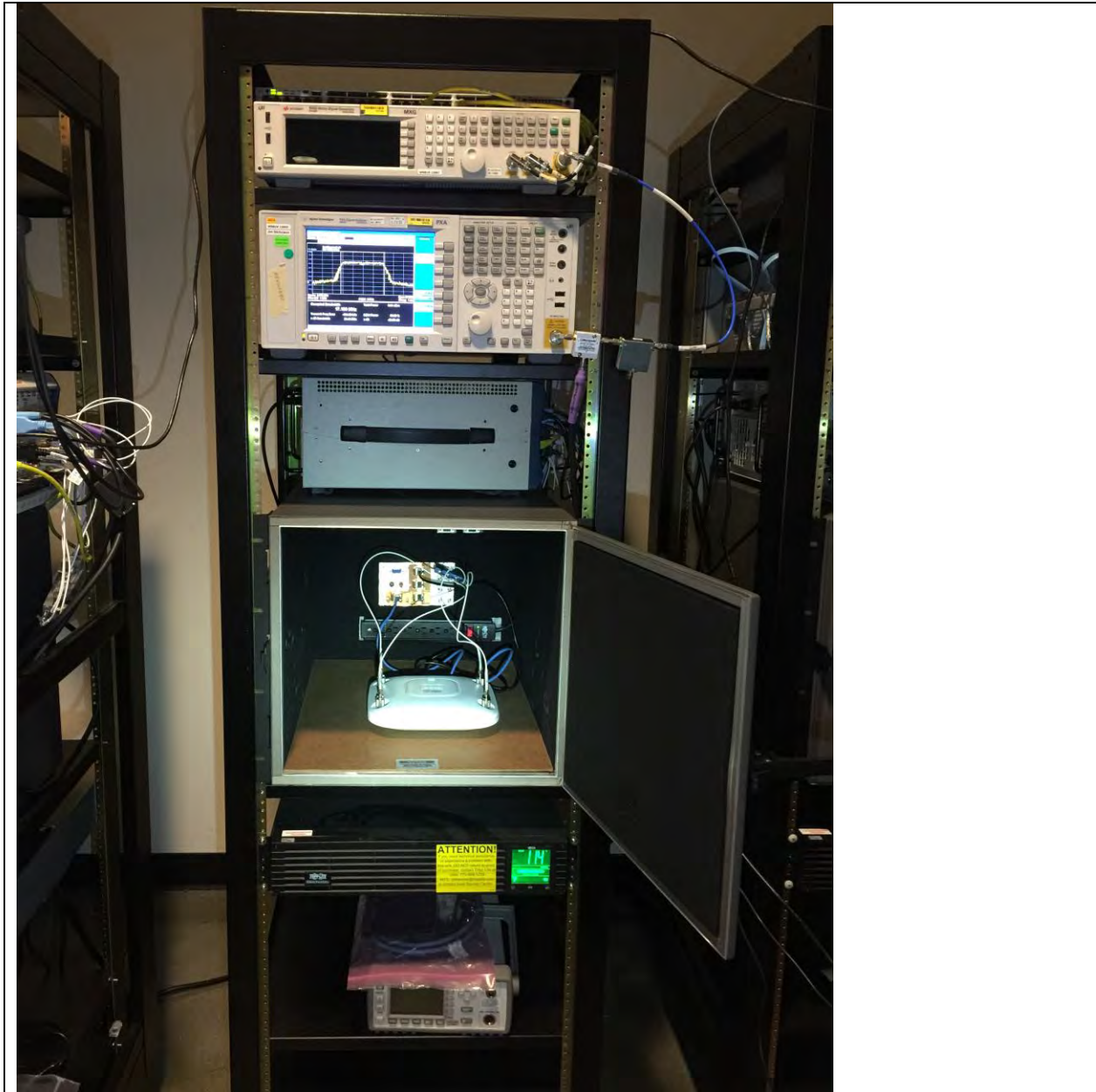
Title: AIR-CAP2602E-B-K9 Physical Test Arrangement Photograph
