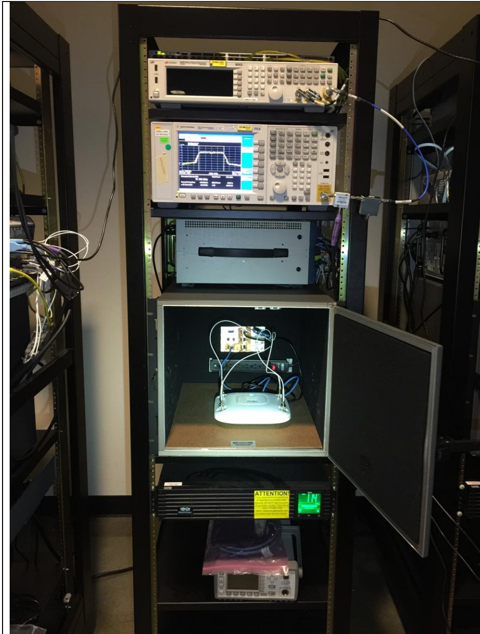
Title: AIR-CAP2602E-B-K9 Physical Test Arrangement Photograph
