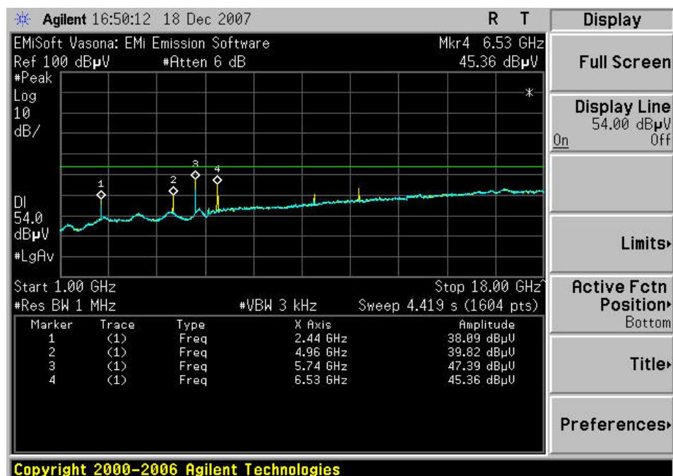
**Radiated Spurious Emissions, 5745 MHz, 24 Mbps, 28 dBm, 17 dBi Antenna
