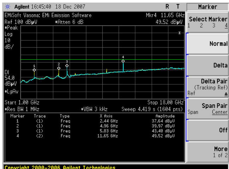
**Radiated Spurious Emissions, 5825 MHz, 24 Mbps, 28 dBm, 17 dBi Antenna
