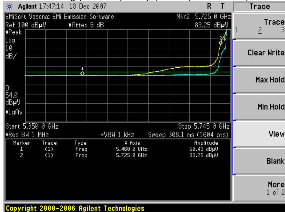
**Radiated Band Edge, 5745 MHz, 24 Mbps, 28 dBm, 8 dBi Antenna, PK**
