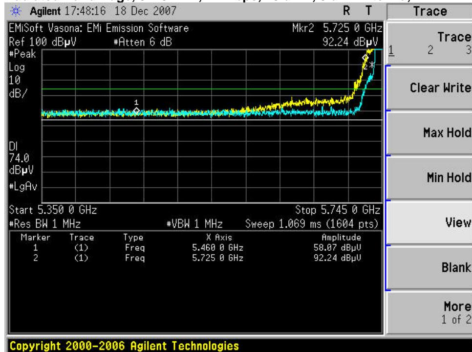
**Radiated Band Edge, 5745 MHz, 24 Mbps, 28 dBm, 17 dBi Antenna, AVG**
