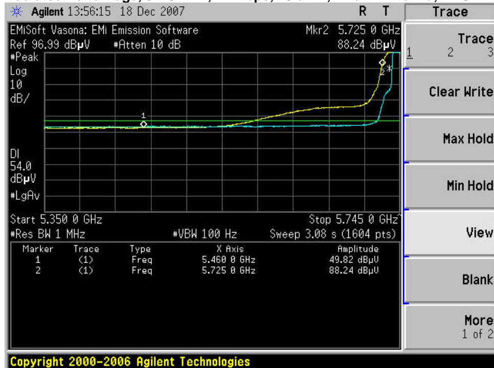
**Radiated Band Edge, 5745 MHz, 24 Mbps, 28 dBm, 17 dBi Antenna, PK**
