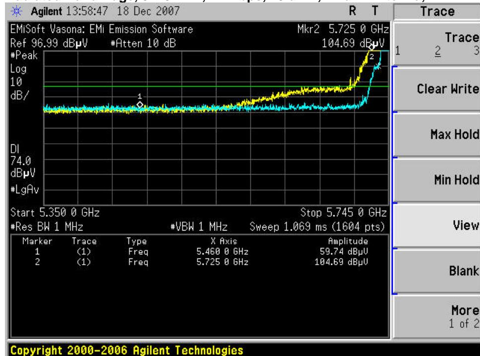
**Radiated Band Edge, 5825 MHz, 24 Mbps, 28 dBm, 8 dBi Antenna, AVG**
