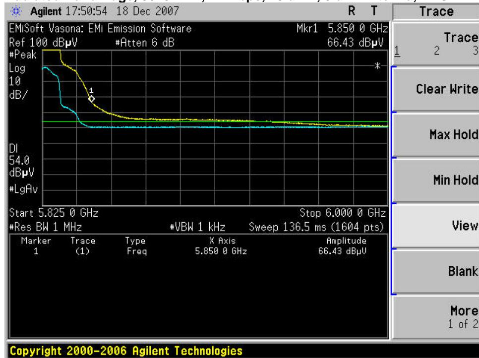
**Radiated Band Edge, 5825 MHz, 24 Mbps, 28 dBm, 8 dBi Antenna, PK**
