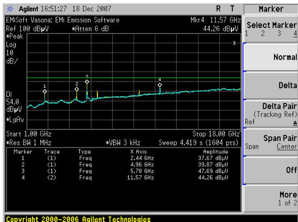
**Radiated Spurious Emissions, 5785 MHz, 24 Mbps, 28 dBm, 17 dBi Antenna
