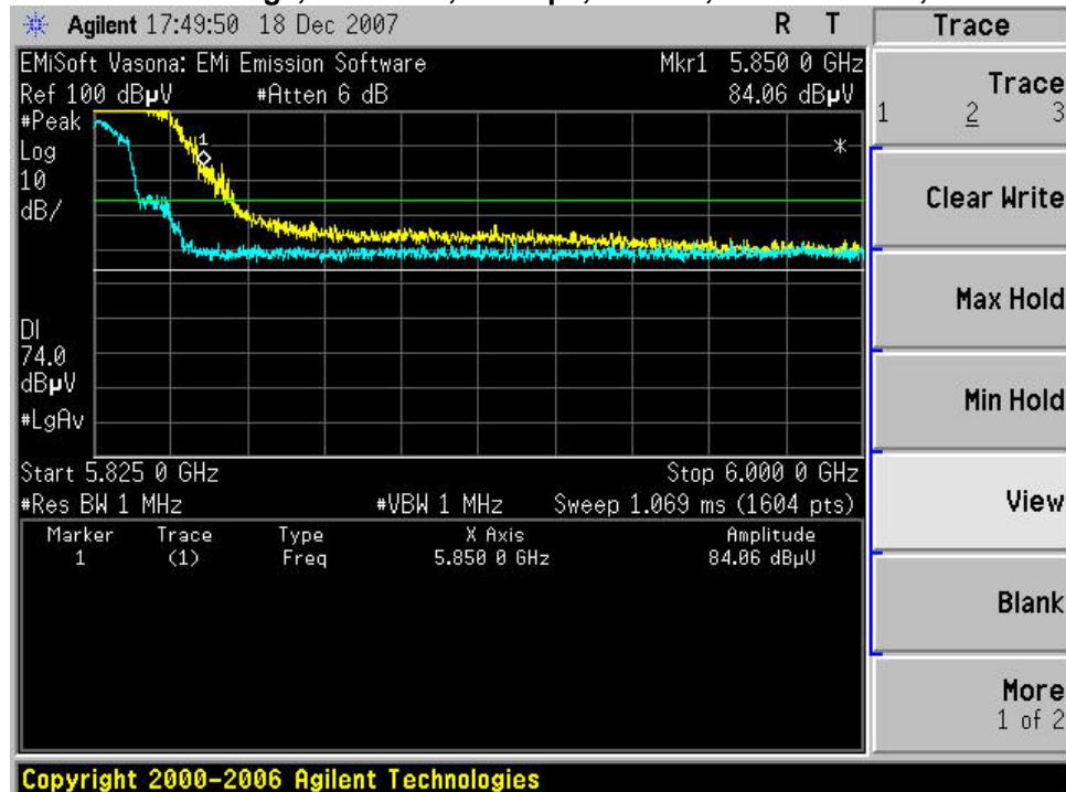
**Radiated Band Edge, 5825 MHz, 24 Mbps, 28 dBm, 17 dBi Antenna, AVG**
