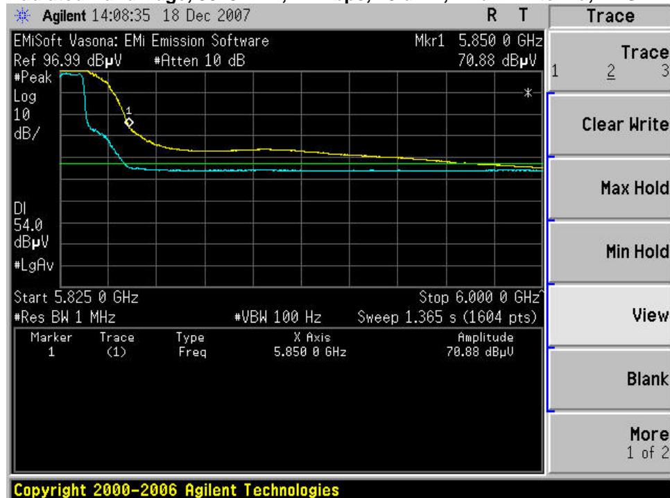
**Radiated Band Edge, 5825 MHz, 24 dBm, 17 dBi Antenna, PK**
