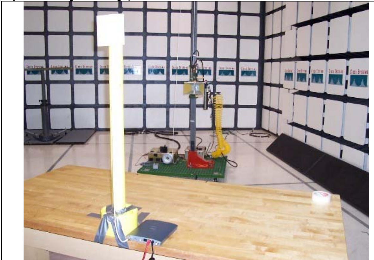
Title: 1-18GHz Radiated Setup, 2.4GHz 9dBi Patch Antenna
