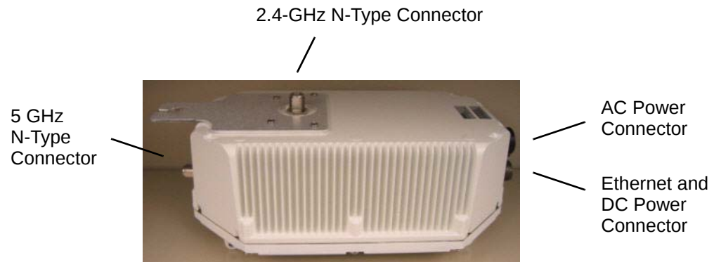
Figure 3-1 Outdoor Access Point Connectors
