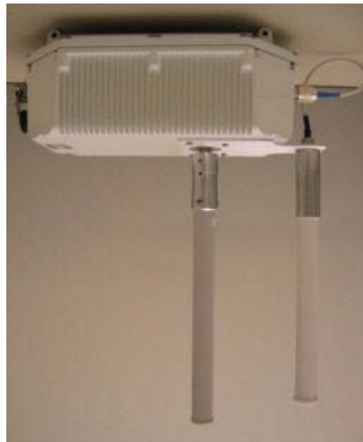
Figure 3-3 Preferred Outdoor Access Point and Antenna Orientation
