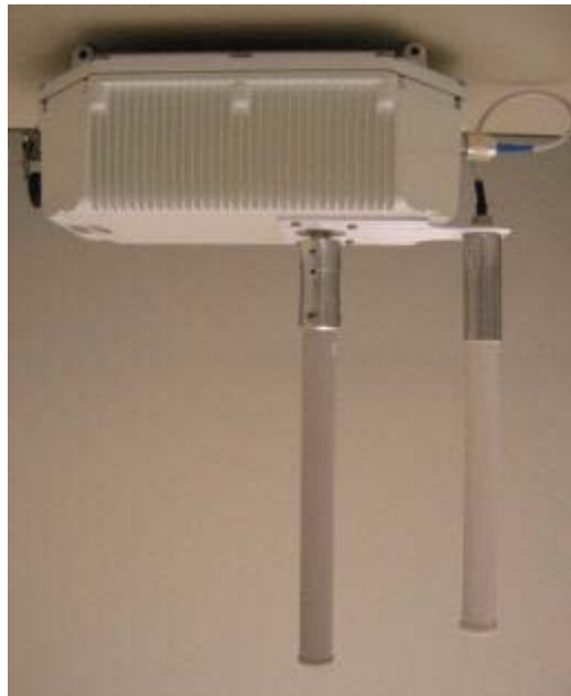
Figure 3-7 Preferred Outdoor Access Point and Antenna Orientation
