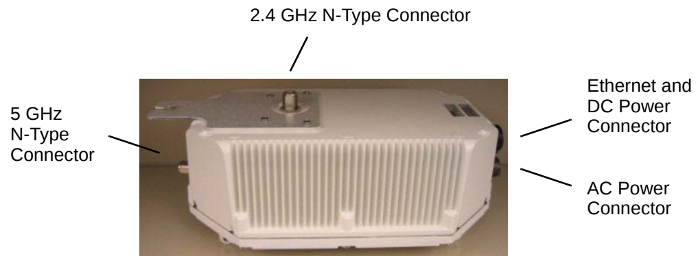
Figure 2-2 Outdoor Access Point Connectors
