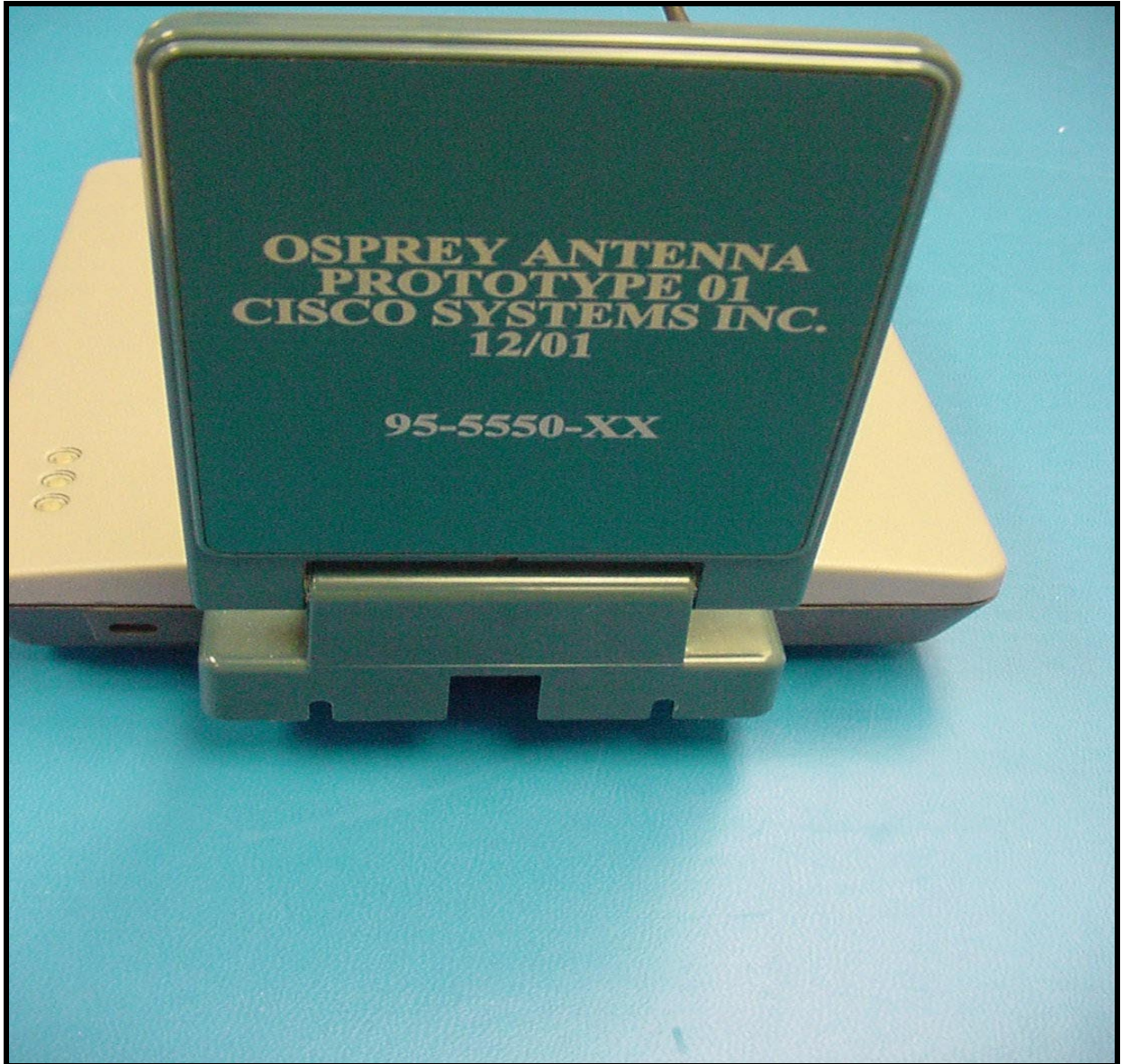
PHOTOGRAPH 6: 5GHZ ANTENNA INSTALLED IN AP1200
