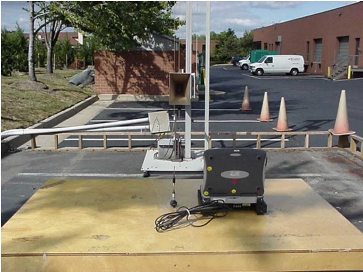
PHOTOGRAPH 4: RADIATED MEASUREMENT REAR VIEW WITH CRADLE (ITRONIX IX250)
